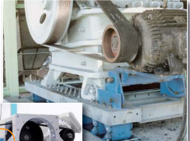
MB 70 drive mount for a jaw-crusher
