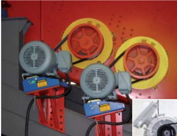
MB 50 drive mounts for a circular-action screen
