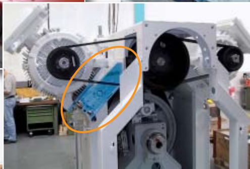
MB 70 drive mounts on a pellet press
