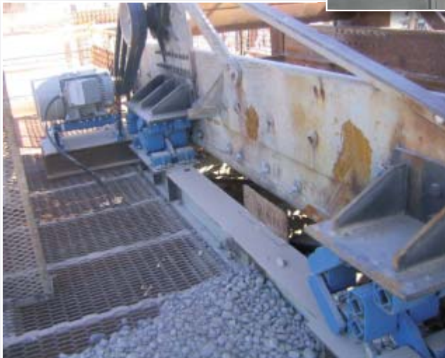
MB 50 drive mount for a linear-action screen
