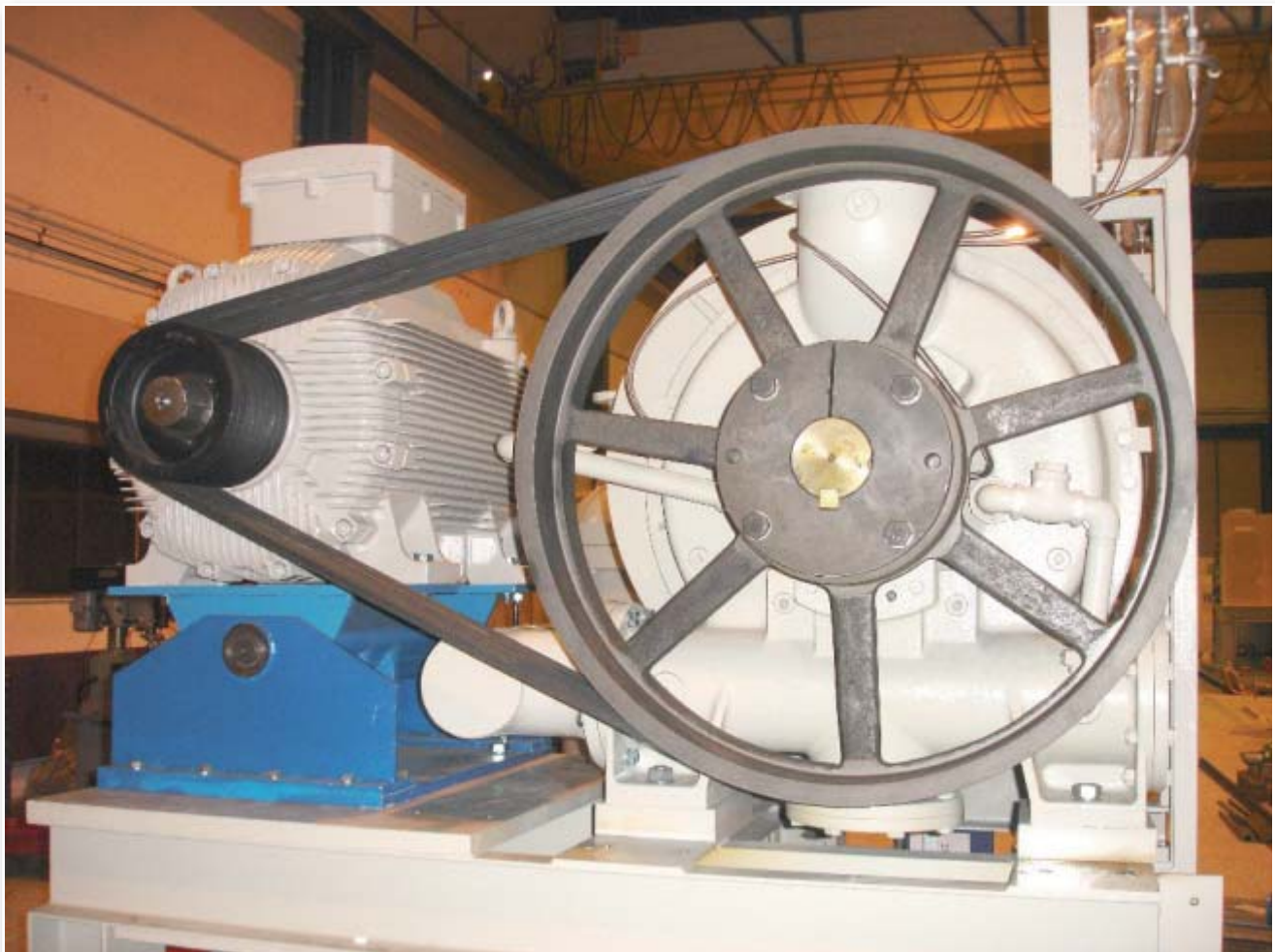
250 kW motor on motorbase MB 100 for a belt drive on a vacuum pump
